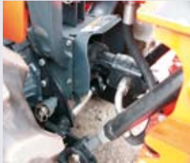
Pump connection to PTO
