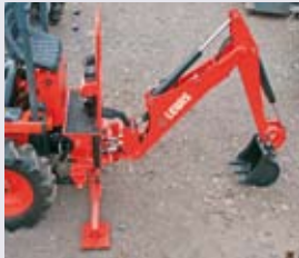
Boom and legs stabilise backhoe
