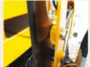
4 Fit loader pins
