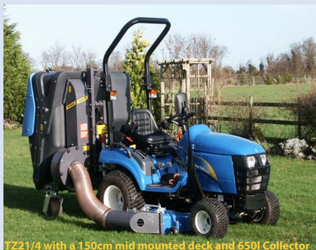
TZ21/4 with a 150cm mid mounted deck and 650l Collector
